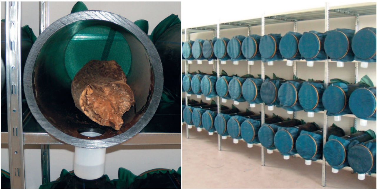
Fig. 1. Left: Ex situ emergence trap. The front screen has been removed to show interior. Right: Storage of the emergence traps used in this study.
